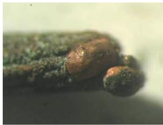
Figure 15. Closer look of the melted cable
