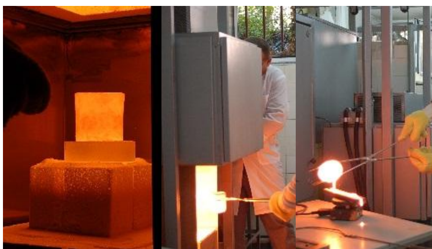
Figure 3. Vitrification of metallurgical waste in chamber furnace
