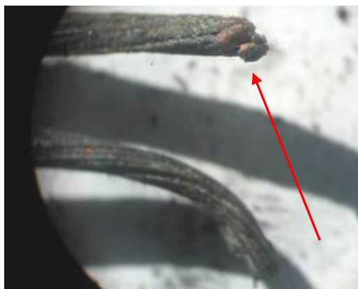
Figure 14. Melted ending of the cable
